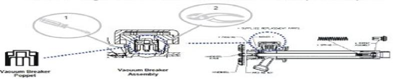
The NIBCO Figure 90 Frost-proof valve (sometimes referred to as a sillcock or hydrant) employs an integral vacuum breaker. The vacuum breaker's function is to prevent any potential siphon effect (via a connected garden hose) in the event of a significant drop in line pressure, thus preventing undesired backflow that could draw contaminants into the potable water supply.
