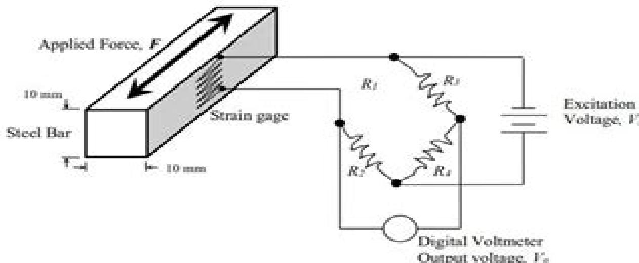
The components taken together represent a force measurement system where the input quantity is force ( $F$ ) and the output quantity is voltage ( $V_o$ ).
