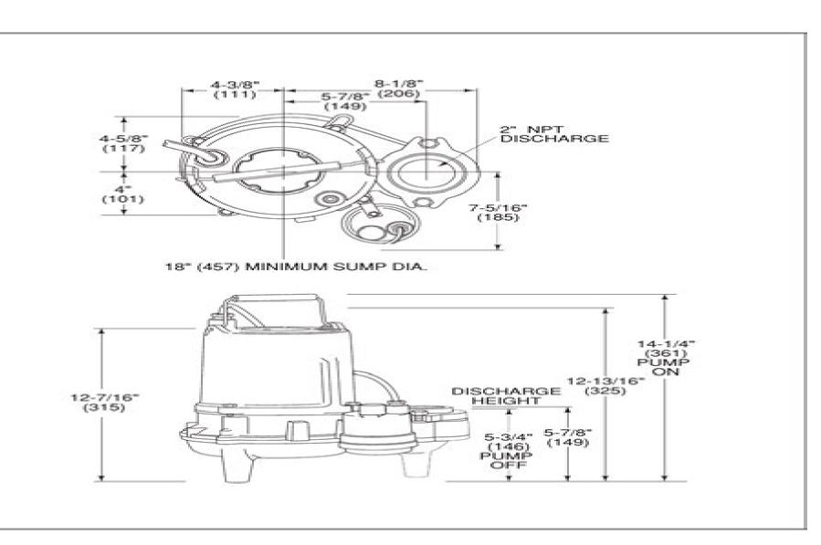
All dimensions in inches. Metric for international use. Component dimensions may vary  $\pm$  1/8 inch. Dimensional data not for construction purpose unless certified. Dimensions and weights are approximate. On/Off level adjustable. We reserve the right to make revisions to our product (s) and the product (s) specifications without notice.
