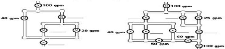
Apply the same principle to fill in the blanks in the following diagrams for charge flow (i.e., current) through a parallel circuit.
