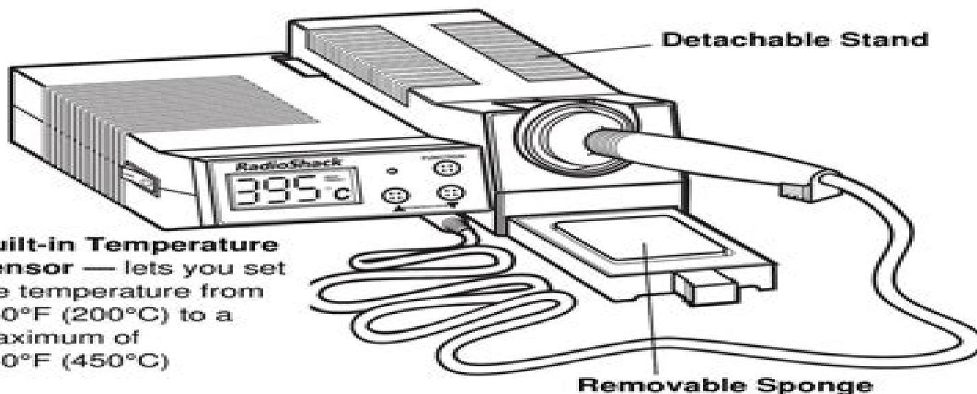
**Built-in Temperature Sensor** — lets you set the temperature from 350°F (200°C) to a maximum of 840°F (450°C)
