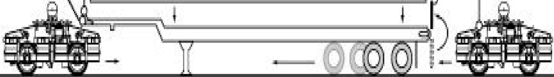
Sliding Tandem provides clearance for RailRunner Bogie
