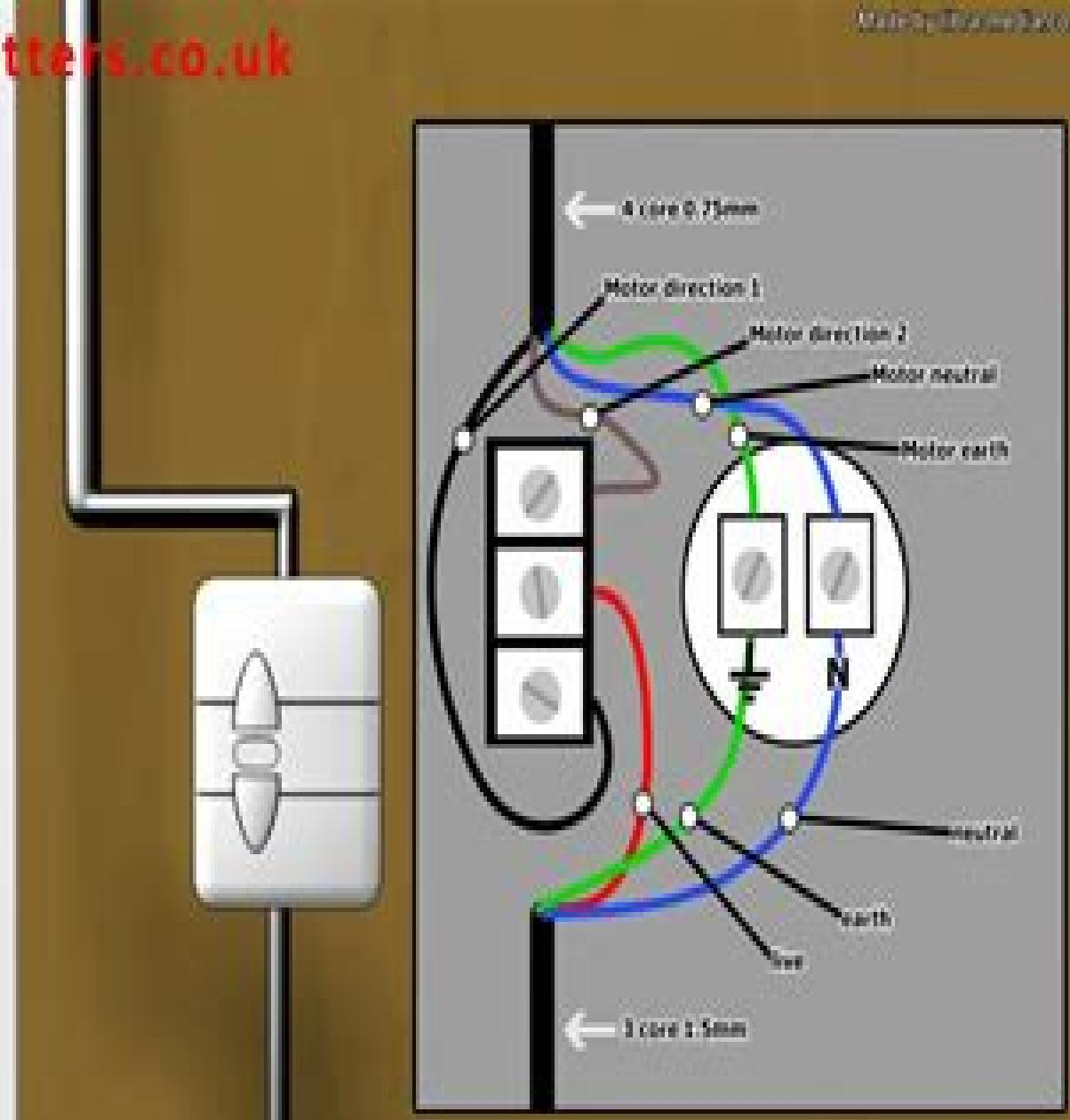
Run the four core motor wire and the three core power supply into the back of the switch. Connect as instructed as per the wiring diagram
