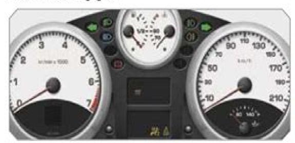
Visual indicators which inform the driver when a system comes into operation (operation or deactivation indicator lights) or of the occurrence of a fault (warning light).
