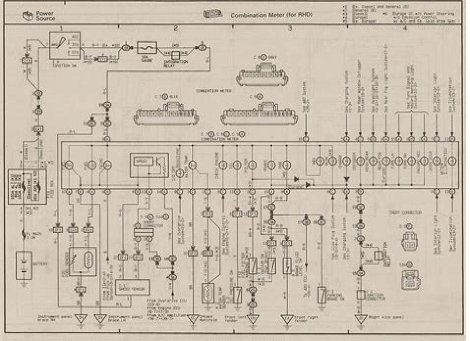
Wiring diagram for instruments
