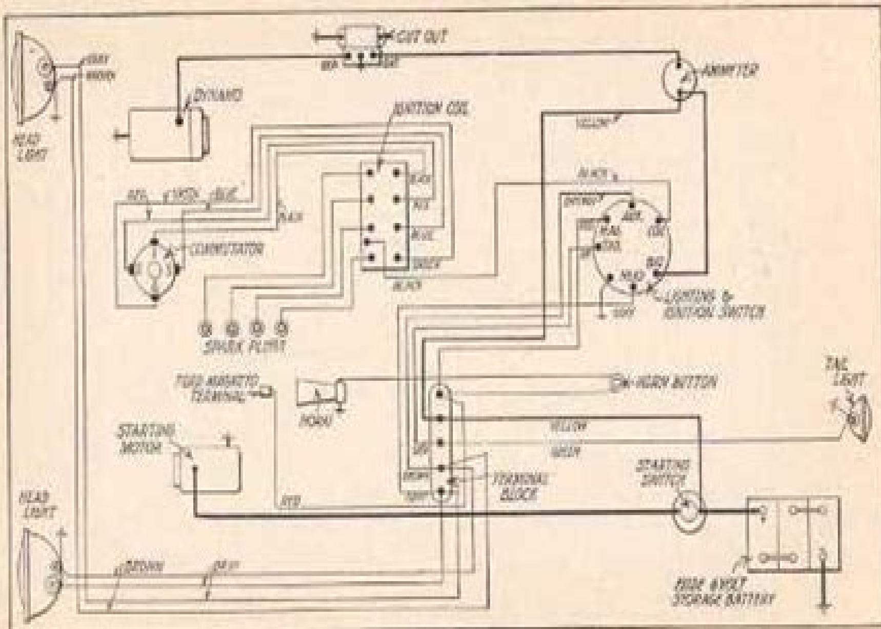
Fig. 17. Wiring Diagram with Cutout on Dash
