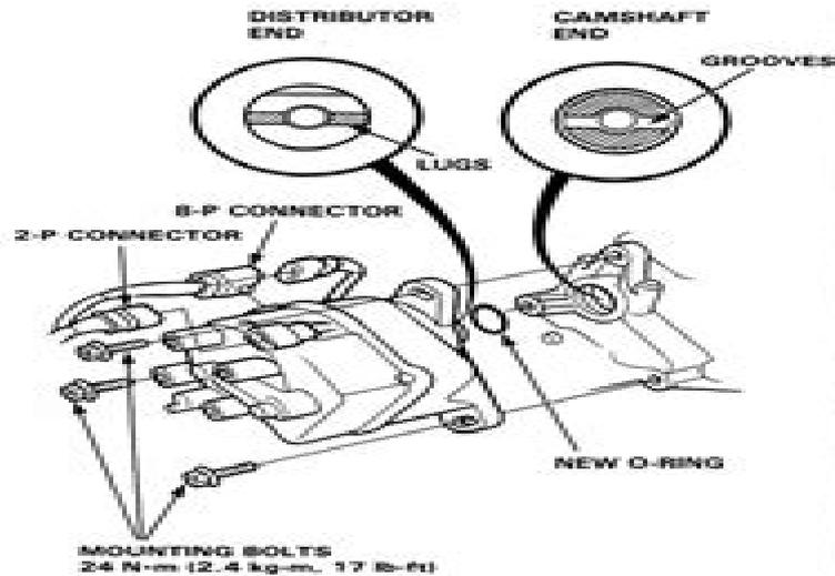
3. Install the mounting bolts and tighten them temporarily.
