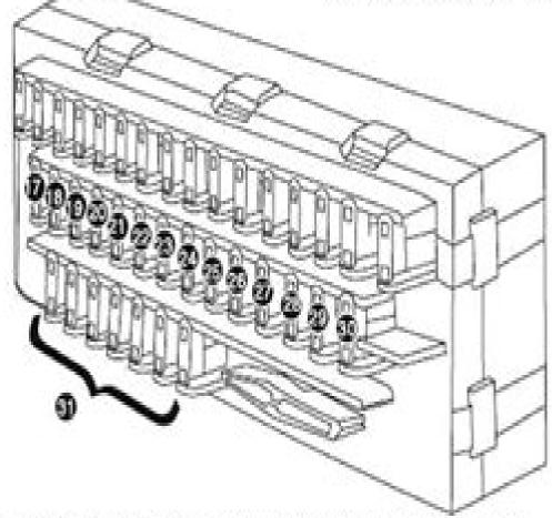
Fuse box is situated under the dashboard to the left hand side of the Driver which included six spare fuses plus special vise for changing fuses. To open the fuse box, pull the cover door of the fuse box forward.
