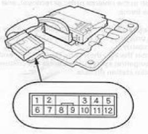
When replacing an equalizer unit connector, match the wires to the cavities as listed in the following table.
