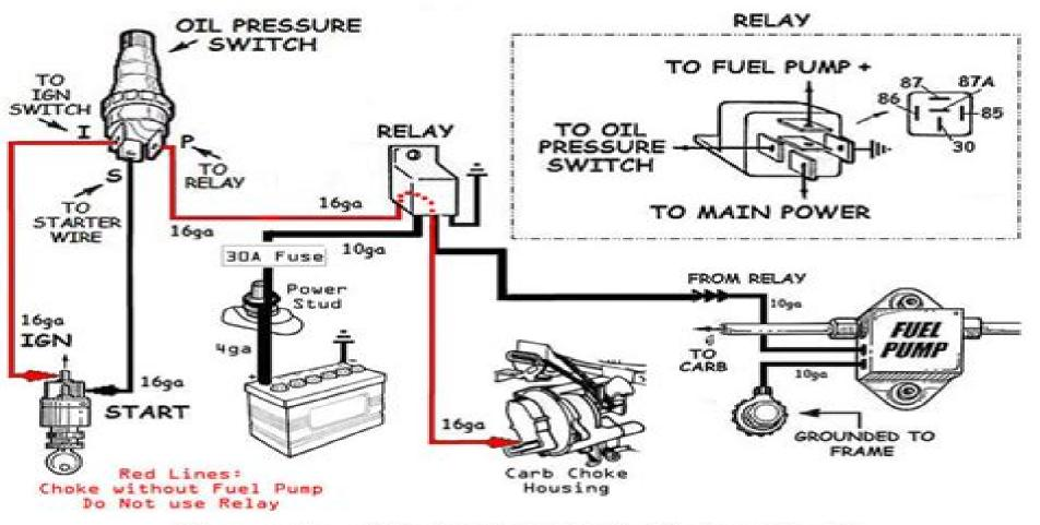
The pressure switch should be installed in the engine oil pressure system at a convenient location. In some instances it may be necessary to install a 'T' fitting below existing oil gauge sender or dash light sender.
