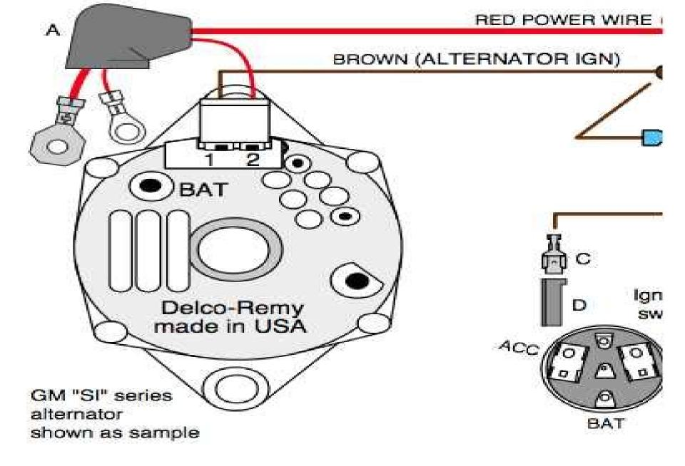
Our Highway 22 instruction sheet illustrates the exciter wire (brown, alternator ign) used for a GM SI-series alternator. This is not needed with a one-wire alternator.
