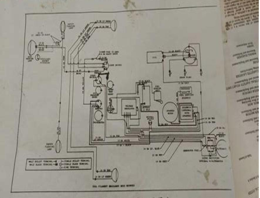
Fig. 40 — Electrical Wiring Schematic (Gas)
