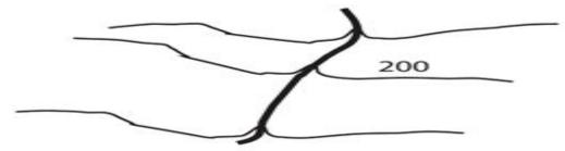
The figure above shows a stream in the center, and three contours crossing the stream. If the contour interval is 50 feet, label the two unlabeled contours.
