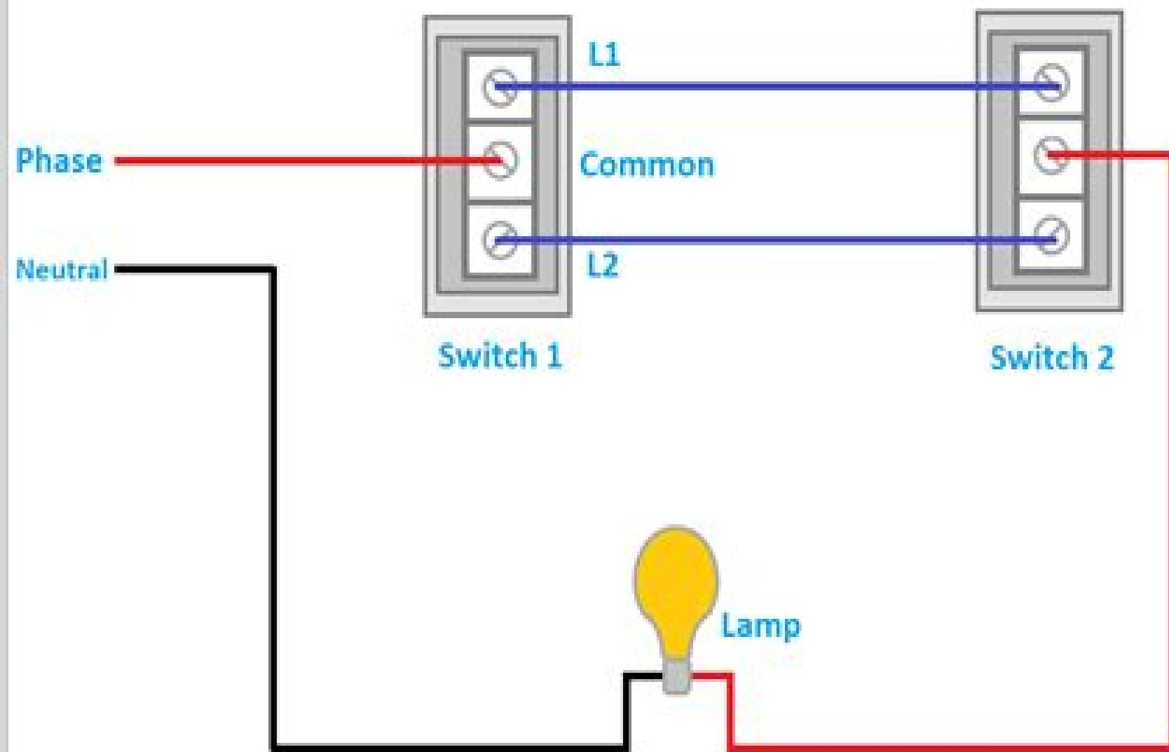
Two Way Switch Connection Diagram : Methode 1
