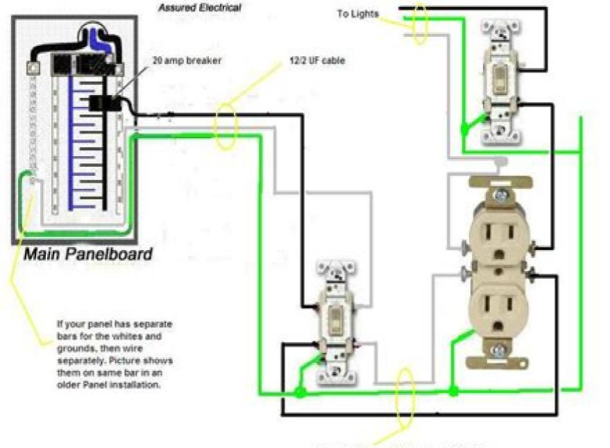
Once inside, run 12/2 romex cable, Uf no longer needed. Receptacles should be GFCI for safety of tools etc.
