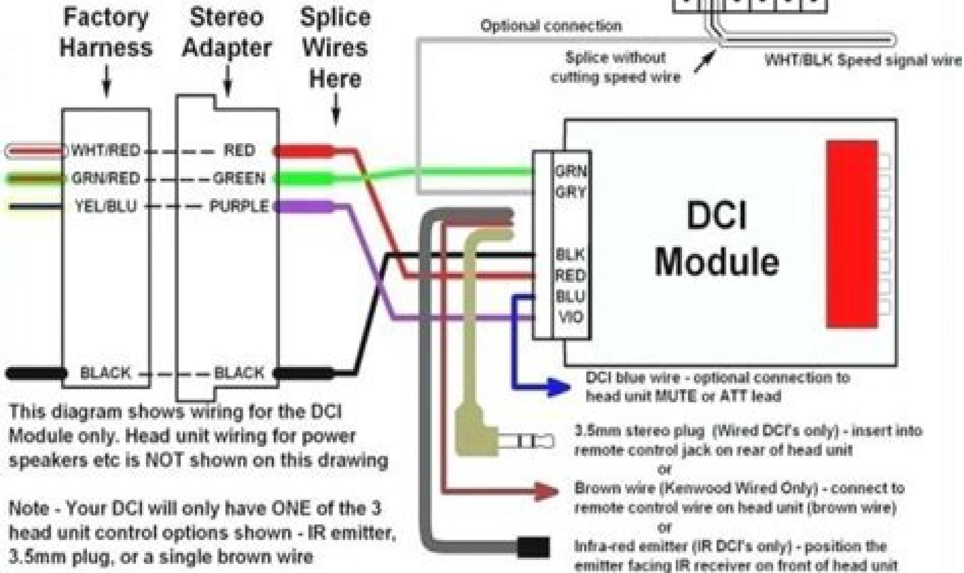
This diagram shows wiring for the DCI Module only. Head unit wiring for power speakers etc is NOT shown on this drawing
