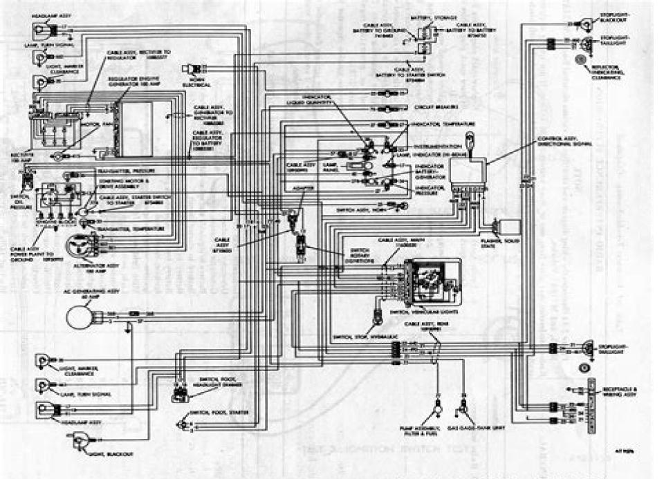
Figure 2-13. Vehicle wiring diagram and cable identification for M151. M151A1. M151A1C. and M718 vehicles.
