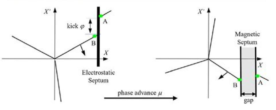
The Electric Septa is thin and delivers a kick to provide a large enough gap that the Magnetic Septa can fully extract.
