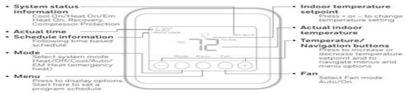
The screen will wake up by pressing any of the five buttons. If powered by the C wire, the screen stays lit for 45 seconds after you complete changes. If powered by battery only, the screen stays lit for 8 seconds. Depending on how your thermostat was installed, the screen light may always be on.
