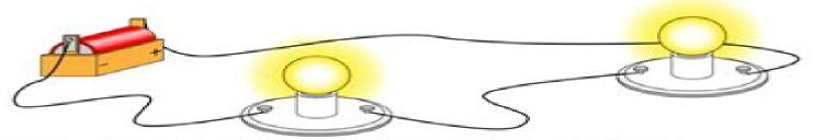
If a light bulb is missing or broken in a series circuit, will the other bulb light? Explain.
