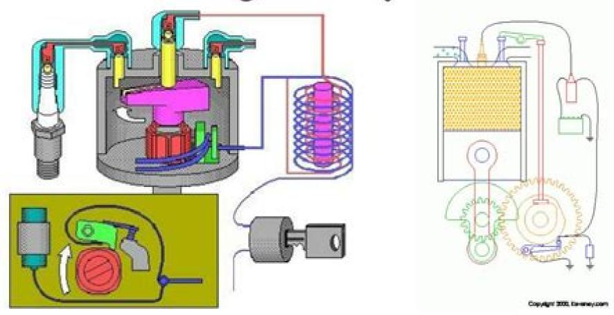
Points are wired in Primary Circuit – When the points are closed, a magnetic field builds in the coil. When the points open, the field collapses and voltage is sent to one of the spark plug.
