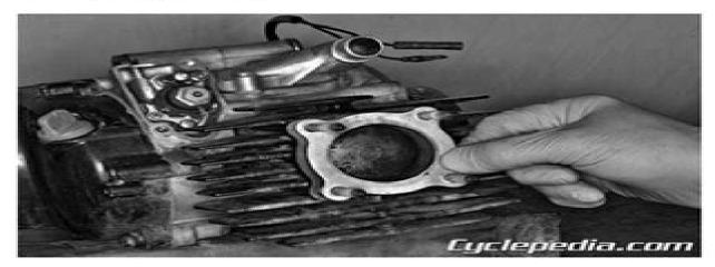
Remove the cylinder head gasket.
