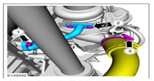
Black arrows are used to draw attention to components (usually fasteners). Arrows with multiples specified (here, x2) identify an identical number of fasteners or items. Callouts (numbers inside circles) show a required sequence or tightening torque.
