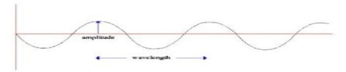
The figure above represents part of a wave. The entire wave can be thought of extending infinitely in both directions. One important characteristics of a wave is its wavelength  $(\lambda)$ , as marked on the figure above.
