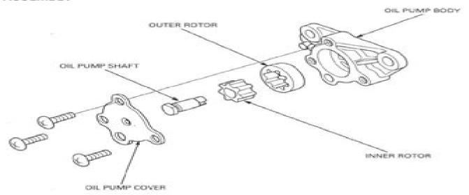
Install the inner and outer rotors into the oil pump body.
