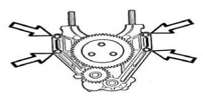
Remove the lubricating oil pump from the main bearing cap. 6
