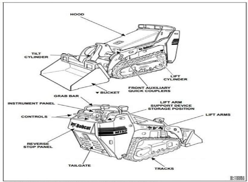
▼ BUCKET - A bucket and other attachments are available for the Bobcat Mini Loader.
