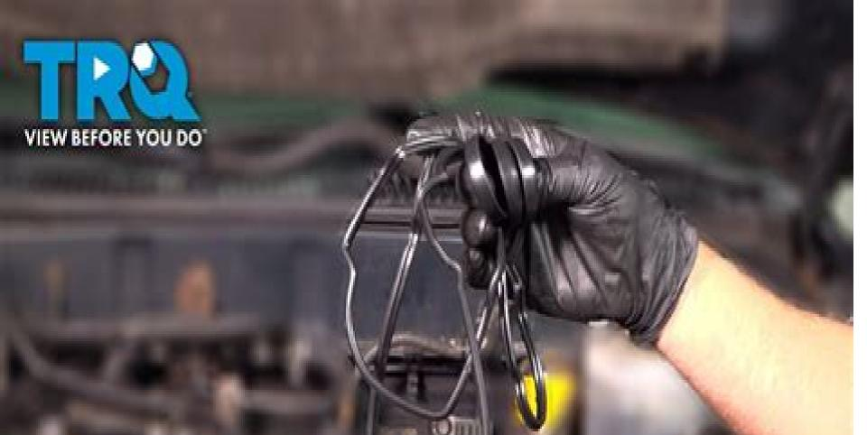
HOW TO REPLACE VALVE COVER GASKETS 1996-2002 TOYOTA 4RUNNER
