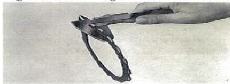
Fig. 6-6-2 Measuring cork plate thickness
