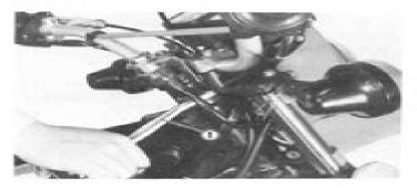
Tighten the bolts following torque.
