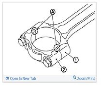
Check that there is no gap in the thrust surface (A) of the joint between connecting rod (1) and connecting rod cap (2) and that these parts are in the correct position. And then, tighten the connecting rod cap bolts.
