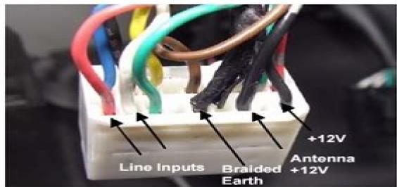
The +12v and Ign 12v may be mixed up. Just double-check these two with a meter.
