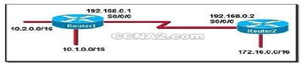
Refer to the exhibit. Router1 and Router2 are running the RIPv1 protocol. The network administrator configures the command network 10.1.0.0 on Router1. What network will Router1 advertise to Router2?
