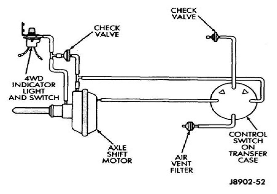
Fig. 87 Command-Trac Axle Vacuum Control System
