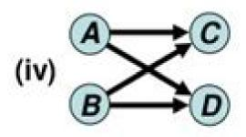
C and D cannot begin until both A and B are completed
