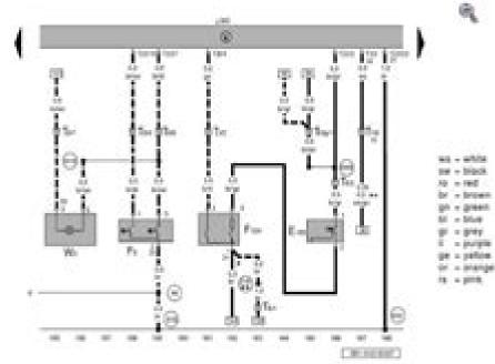
Convenience system central control unit, rear lid central locking and luggage compartment light for Variant, lock cylinder contact switch
