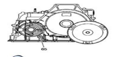
The oil level control plug (65) is located on the torque converter side of the transmission.
