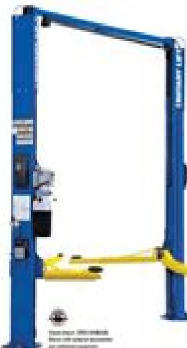
Three-stage, asymmetrical lift arm design allows maximum lift height.
