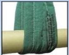
Sling users must take the slack out, before lifting.
