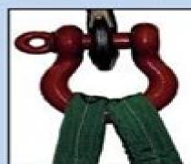
When placing multiple Twin-Path\* slings in hardware, place the slings directly on top of each other or side by side. DO NOT stair-step paths partially over each other.
