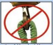
Keep folds and wrinkles off the hook, hardware and/or load.
