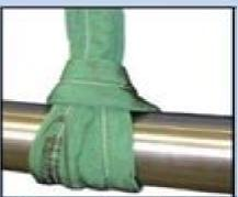
Make sure the paths of the sling run smooth in the bite of the choker hitch without twisting.
