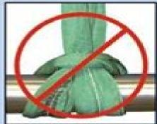
DO NOT allow the sling to roll over itself and twist at the bite of the choker hitch.
