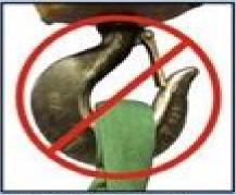
DO NOT fold one path over the other path to make the sling "fit".
