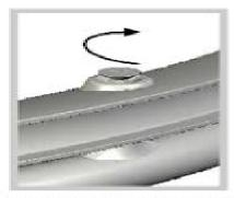
Place the bolts and the bolt caps (x6) through the Loopwheel and down into the push rim. Screwthe bolts into place using a 'posi-drive' screw driver, to a torque setting of 5 N/mm. (Option to thread lock the bolts in place)
