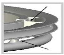
Place the Loopwheel onto the 'push rim spacers', making sure the wheel is orientated so that the 'rib' on the 'rim connector' is on the opposite side to the push rim.
