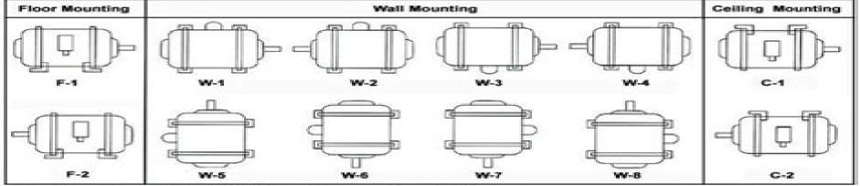
Note: Assemble symbols F-1, W-2, W-8 and C-2 mean the conduit box, the mounting feet and the shaft-extension are at the same location.
