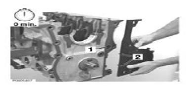
4 Install a new O-ring (1) Install the side plate. Take care to ensure that the sealant is not scraped off during installation. Torque the bolts (2) to 25 Nm (18 lbf ft).
