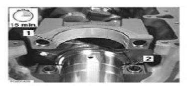
6 Lift the crankshaft into place install the main bearing caps. Make sure the bearing shell looking tabs (1) and (2) are aligned as illustrated. The main bearing caps are numbered 1–5 (D4) or 1–7 (D6). Number "1" must be installed furthest forwards (close to the oroulation pump.)
