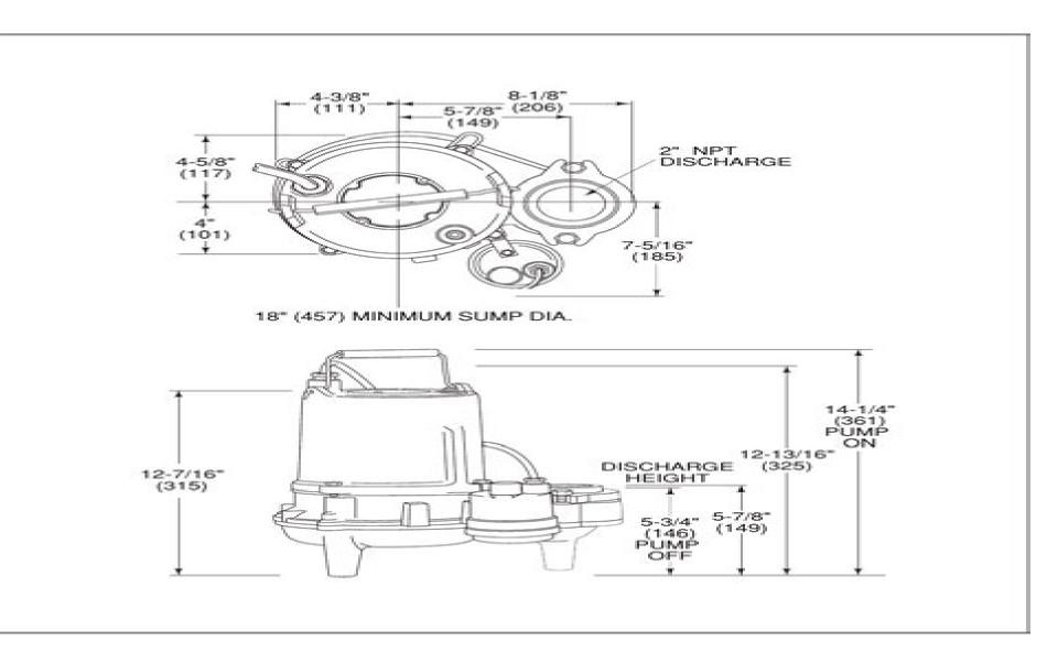
All dimensions in inches. Metric for international use, Component dimensions may vary  $\pm$  1/8 inch. Dimensional data not for construction purpose unless certified. Dimensions and weights are approximate. On/Off level adjustable. We reserve the right to make revisions to our product (s) and the product (s) specifications without notice.
