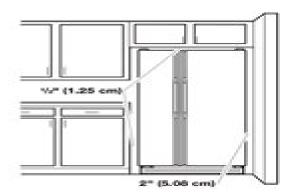
To ensure proper ventilation for your refrigerator, allow for 1/2" (1.25 cm) space on each side and at the top. When installing your refrigerator next to a fixed wall, leave 2" (5.08 cm) minimum on each side (depending on your model) to allow for the door to swing open. If your refrigerator has a water dispenser and ice maker, allow extra space at the back for the water line connections.
