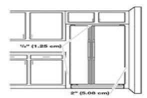
Normal minimum cabinet cut-out width required for product installation is 36° (91.4 cm). However, if the product is placed against an extended wall and the ability to remove the crisper pans is desired, an additional 18° (45.7 cm) of cabinet width is required, so a total cabinet opening width of 54° (137.2 cm) is recommended.
