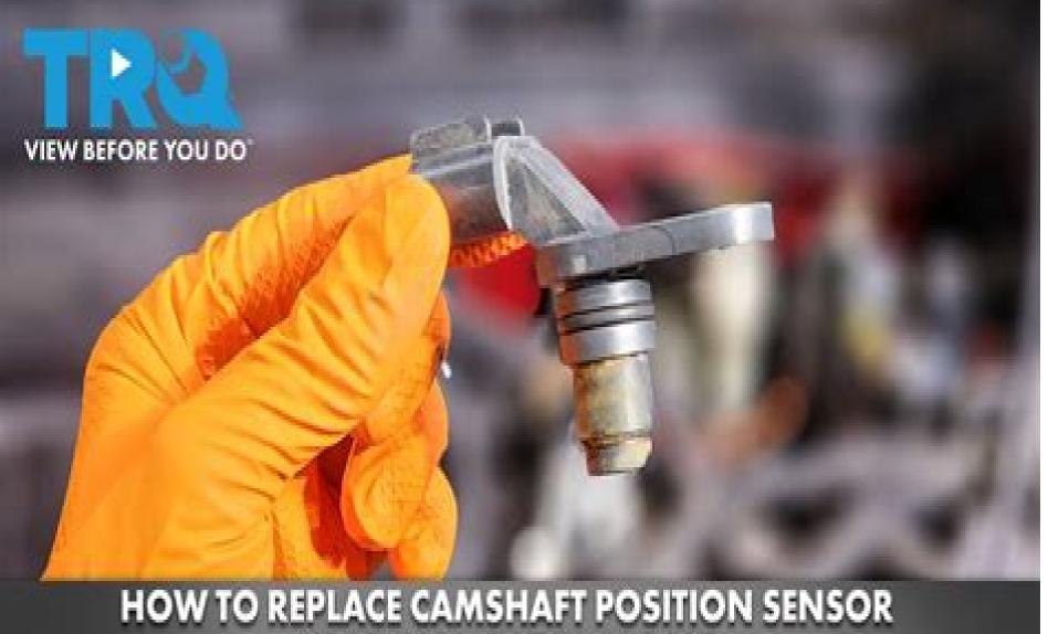
HOW TO REPLACE CAMSHAFT POSITION SENSOR 2005-2010 CHEVY COBALT
